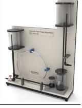
The apparatus can be used to demonstrate the creation and outcome of water hammer and to study how a hydraulic ram works. The water is fed to the ram via a long pipe at a gradient.
